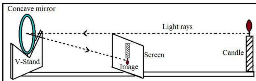
**Procedure:-** 1. Place the concave mirror on V-stand, a candle and meter scale as shown in figure.
