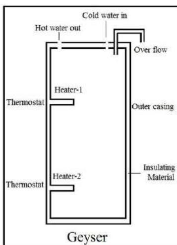
**Working of Geyser:** - 1. Geyser is an electrical device which converts the electrical energy into heat energy.
