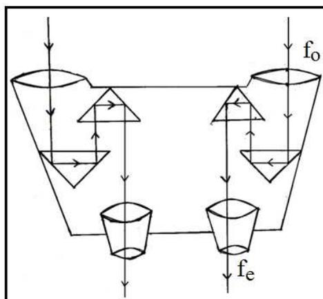
1. If two telescopes are mounted parallel to each other so that an object can be seen by both the eyes simultaneously the arrangement is called binocular.
